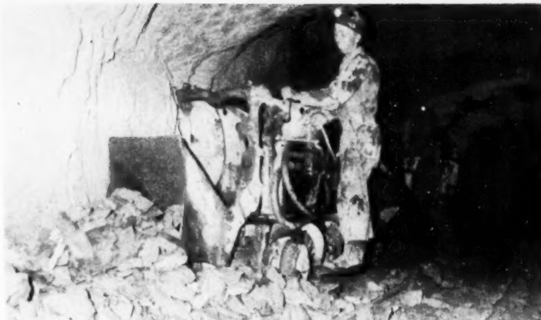
Ray Caspar operates an Eimco 12-B Rocker Shovel in 1502-N crosscut. This crosscut will provide for high-speed double-track haulage from the Mayflower fissure, and single-track haulage from the Pearl fissure to the Mayflower.
